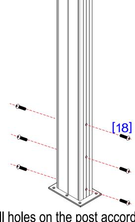
Drill holes on the post according position of the base plate hole
