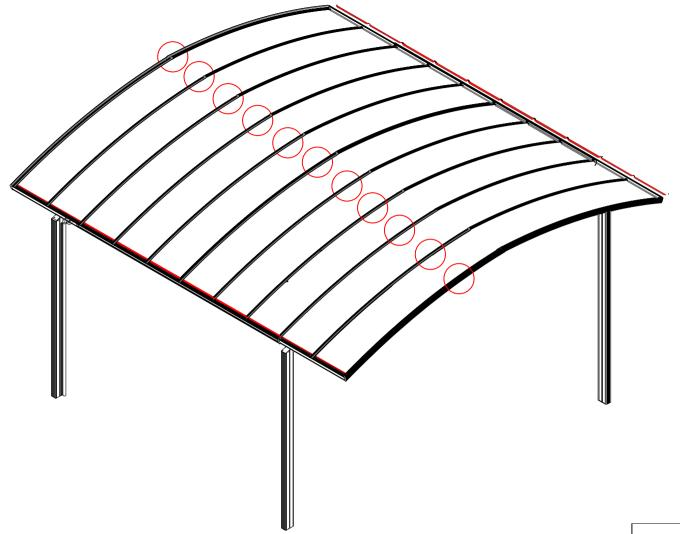
According to the previous method, install the solid pc board in sequence, and then install the cover linear
